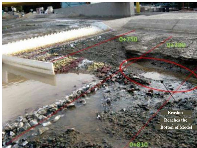
Figure 6. Critic Erosion presented at the Physical Model with unprotected bed (1000 Years Flow)
