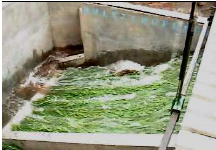
Figure 2. Failure at a 35 L/s/m unit discharge using grass mats of Pennisetum clandestinum.
