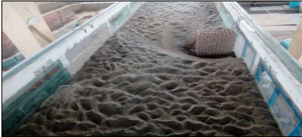
Figure 6. View of the flume bed after a test. Notice bedforms and scour pattern around the ELJ groyne
