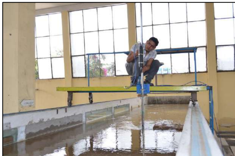
Figure 5. Velocity field data acquisition using an ADV profiler near the ELJ groyne. This photograph was taken looking in the downstream direction.
