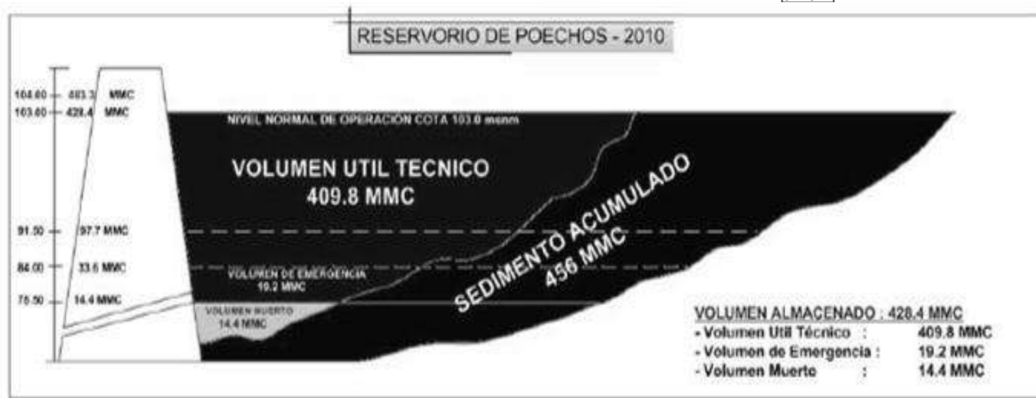
Figure 1 Volume of Poechos reservoir. Left, design volume in 1978. Right, useful volume in 2002. Down, useful volume in 2010.
